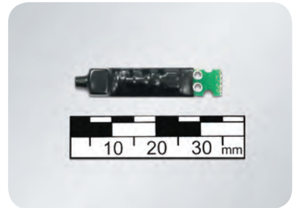
ENPM 010 with heat-shrink tubing covering
